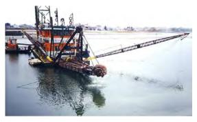
articulated "arms" and hydraulic pumping to remove the material from the channel bottom and place it in a hopper in the center and bow of the vessel. The dredged sediments were deposited in a near shore area off Wells Beach, about 5,000 feet south of the dredge site. The dredged material is intended to function as a feeder berm, providing a sand source for nourishment of the beach.
